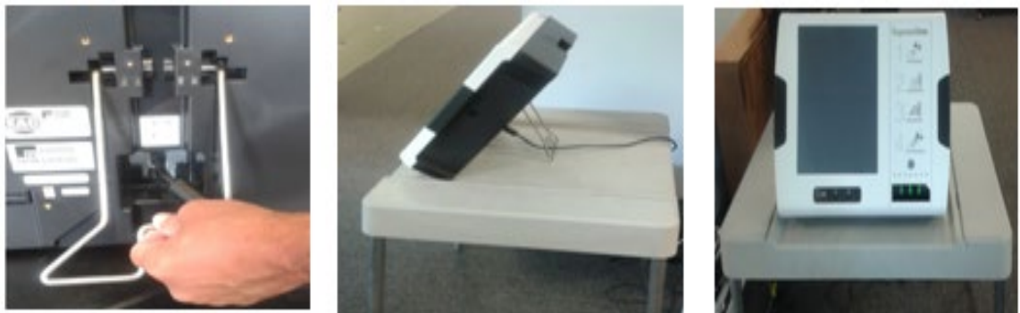
Figure - Setting Up the Ballot Marking Device
