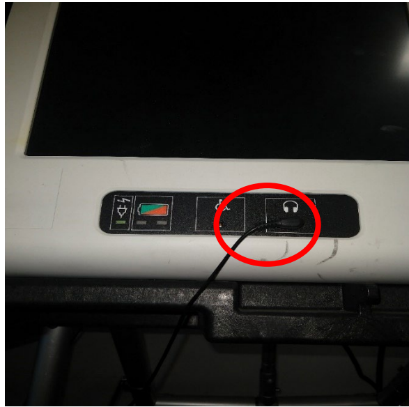
Figure - Headphones Plugged in to the Audio Port of the Ballot Marking Device
