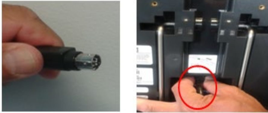
Figure - Small Circular Plug in the Port of the Ballot Marking Device
