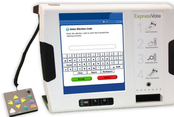
Figure - Election Code on the Ballot Marking Device
