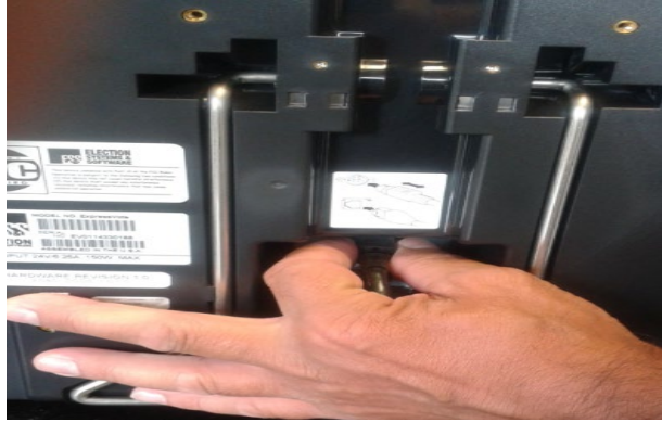
Figure - Power Cord on the Back of the Ballot Marking Device
