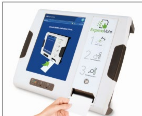
Figure - Slanted Corner of the Card to the Top Right of the Ballot Marking Device
