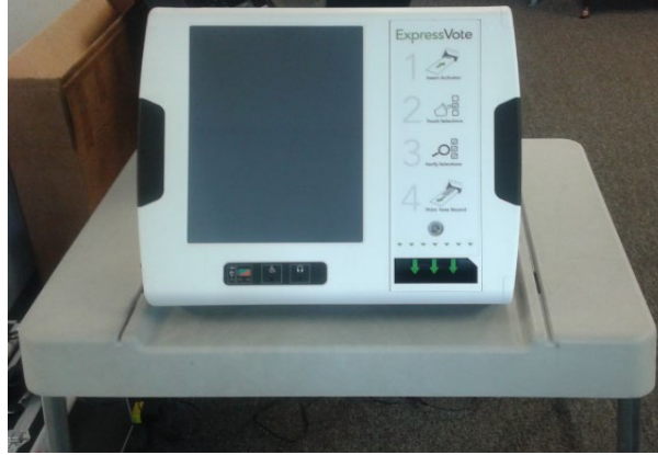
Figure - Removed Privacy Screens of the Ballot Marking Device
