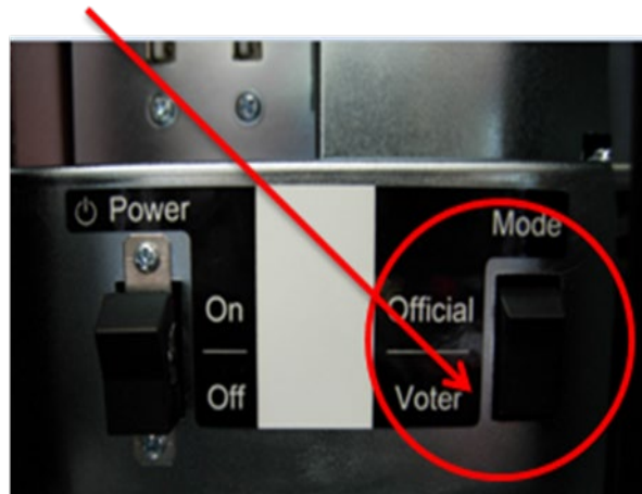
Figure - "Mode" Switch is on "Voter" of the Ballot Marking Device
