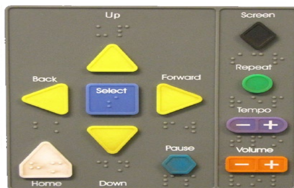
Figure - Keypad of the Ballot Marking Device
