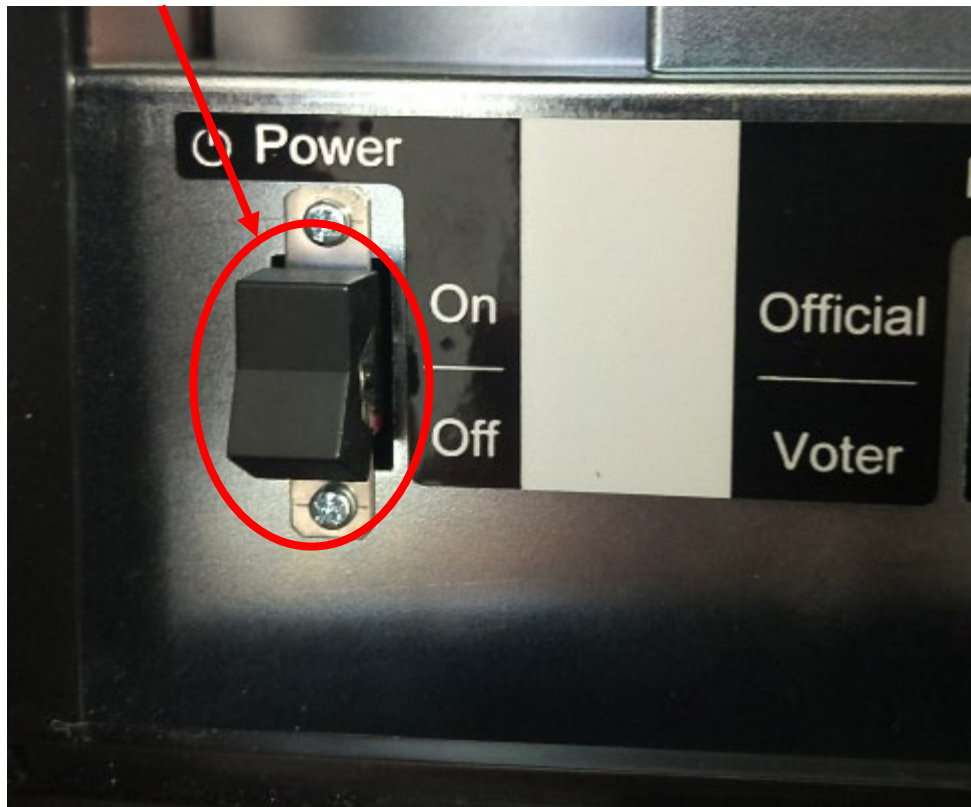
Figure - "Power" Switch to the "On" Position of the Ballot Marking Device
