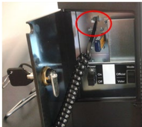
Figure - Keypad Plug of the Ballot Marking Device
