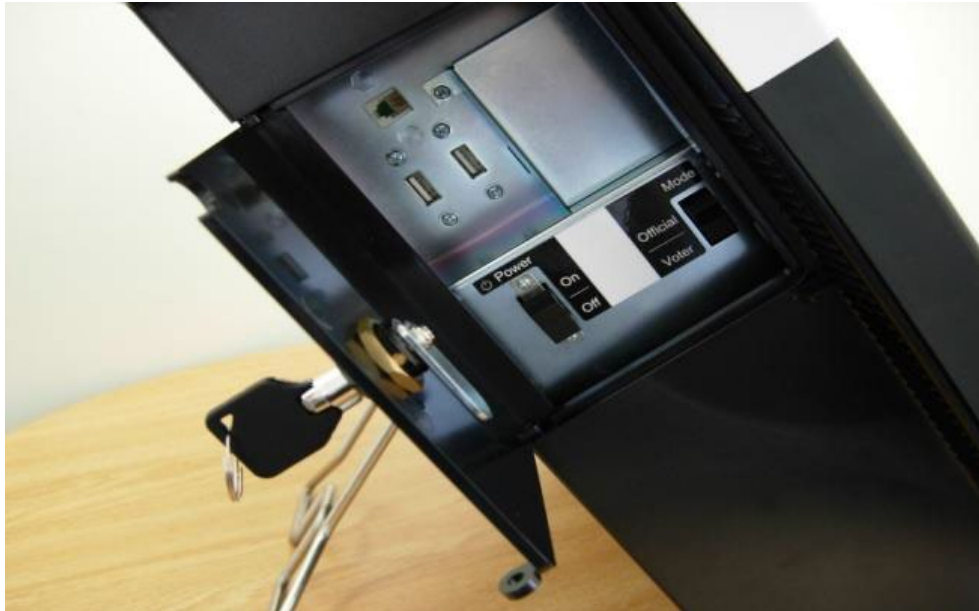
Figure - Side Compartment Door of the Ballot Marking Device
