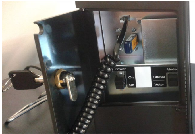
Figure - Opened Side Compartment Door of the Ballot Marking Device
